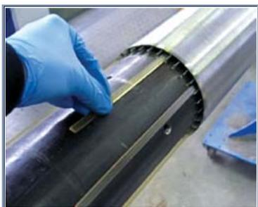
Fig. 2. Tracer-impregnated matrix strips being inserted into a sand screen.<sup>47</sup>
